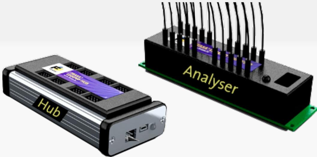
The Feasa™ LEGEND is a test solution for applications with large LED counts. The Feasa™ Legend system consists of two component parts, a Hub and a Satellite Analyser. The Hub can be mounted in the Test Station or in the Test Fixture and can control up to 8 Satellite Analysers. Each Satellite Analyser can test up to 20 LEDs so a fully populated Hub can test up to 160 LEDs concurrently.
