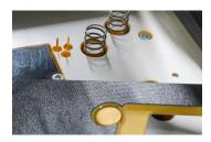
A 'start switch' (internal: 3-pin connector) is installed in the ME2 as standard. This contacts a brass plate on the moving plate. This allows the 'fixture down' signal to be queried during ICT. Also possible with bi-level: In addition to ICT, there is also the FKT query. The ESD needles (long stroke!) contact the moving plate on the underside of the plate in each fixture. The underside is connected to the top side in an ESD dissipative manner by means of a so-called Tapex socket and a screw.
